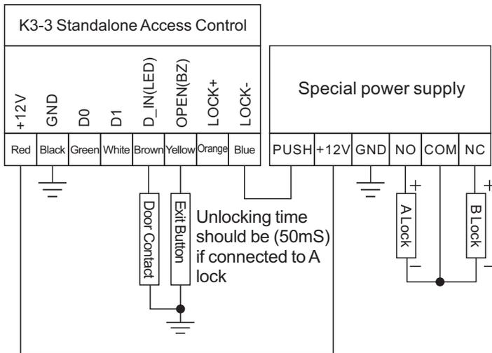
Wiring diagram (Special power supply for access control)
