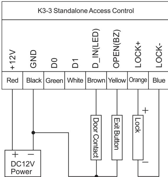
Wiring diagram (DC 12V power supply)
